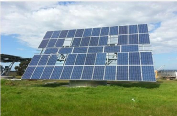
The solar array tracks the sun throughout the day, increasing annual output by more than 30% compared to a fixed north facing solar PV system. This system produces more than 100,000kWh each year – enough to power more than 13 average homes.
